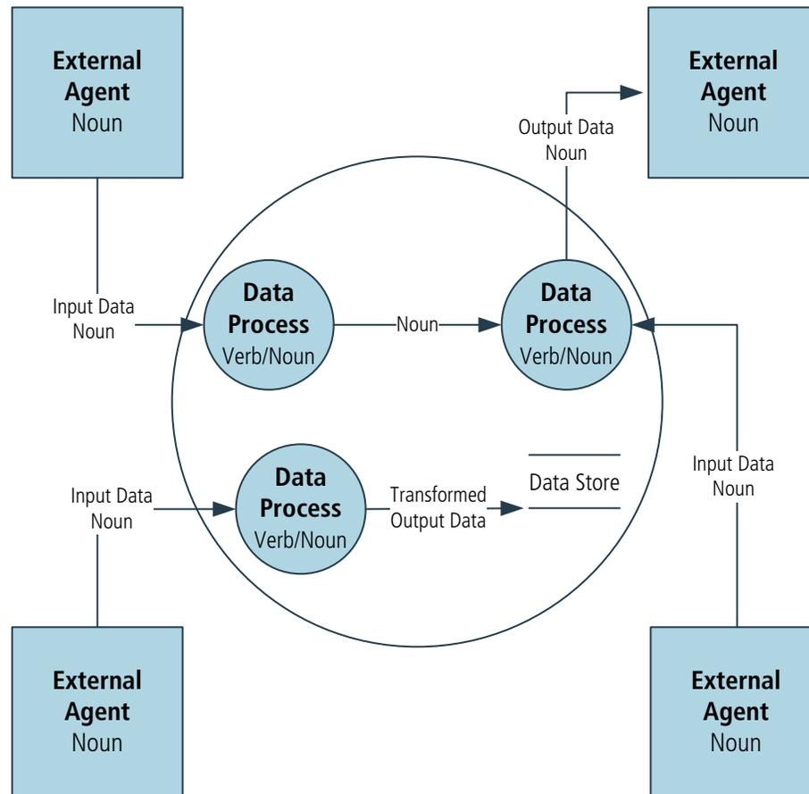
Further levels of the data flow diagram (level 2, level 3 and so forth) break down the major processes from the level 1 diagram. Level 1 diagrams are useful to show the internal partitioning of the work and the data that flows between the partitions, as well as the stored data used by each of the partitions. Each of the partitions can be further decomposed if needed. The externals remain the same and additional flows and stores are defined.
