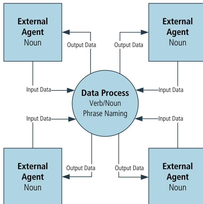
The next level of data flow diagrams is the level 1 diagram. Level 1 diagrams illustrate the processes related to the system with the respective input data, output transformed data, and data stores.
