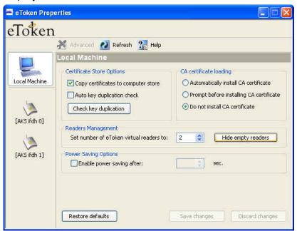
Below the **Local Machine** button (left panel), are buttons which represent eTokens and/or smartcard readers available on the system. When installing the eToken RTE, two virtual smartcard readers are installed with it. The names of eToken smartcard readers begin with **AKS ifdh**. This is followed by the reader number.
